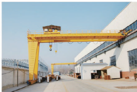
MGB double-girder semi-gantry crane with hook
