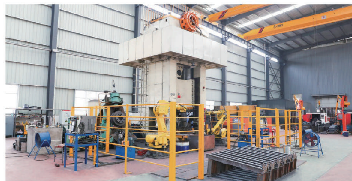
车轮锻造碾压复合工艺智能化流水线 Intelligent assembly line of wheel forging and rolling composite process
