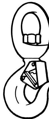
Fig. 10-1.1-11 Self-Closing Flapper Latch (Swivel Hook)
