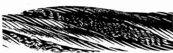
Local increase in diameter of Lang lay wire rope
