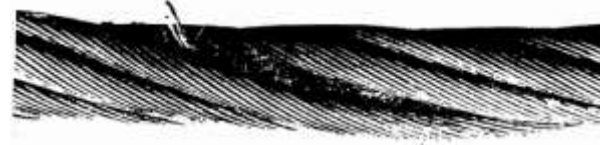
Local increase in wire rope diameter
