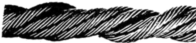
Localized reduction in diameter
